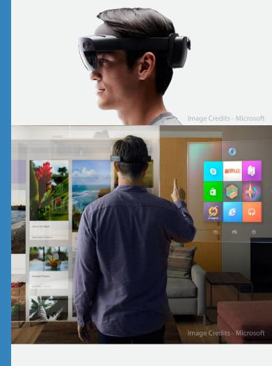
Currently on its second iteration, HoloLens 2 is an Augmented and Mixed Reality headset and is described by the tech giant as a "fully untethered, see-through holographic computer", allowing users to experience 3D content as if part of their physical environment.
